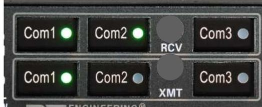
When switching from COM 1 to COM 2, while COM 2 audio had been selected, Com 1 audio will continue to be heard. This eliminates the pilot having to switch Com 1 audio back on, if desired.
