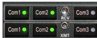
Split mode is possible with pilot on Com 1, copilot on Com 2 or 3. Pilot on Com 2 or Com 3 and Copilot on Com 1 is not possible.
