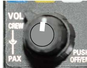
Adjust the radios and intercom volume for a comfortable listening level for the pilot. Most general aviation headsets today have built-in volume controls; therefore, passenger volume can be adjusted at the headset.
