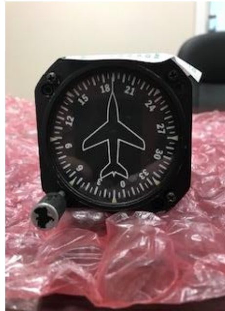
RC Allen - Directional Gyro – Model RCA11A-8 (Serviceable) $1500 OBO
